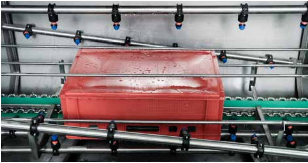
High-alloy stainless steel conveyor chains: Outstanding resistance to heat and moisture as well as corrosion, even if aggressive cleaning agents are used.
