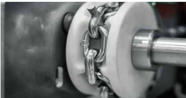
Electropolished surfaces will largely repel flash rust and contamination, and ensure that the chain runs smoothly over the pulleys.
